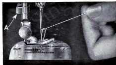
Fig. 16. Drawing up Bobbin Thread
